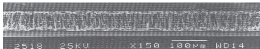
MICROGRAPHS VIEW OF ETCHED ALUMINIUM FOIL
