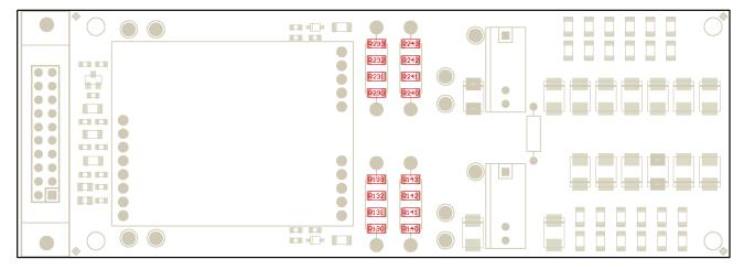
*Fig. 4: Assembly drawing of 2BB0108T with highlighted SMD gate resistors Turn-on gate resistors: R140...R143, R240...R243 Turn-off gate resistors: R130...R133, R230...R233*
