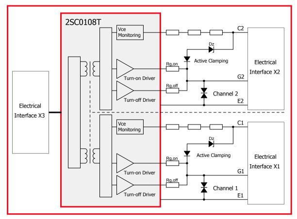
The basic topology of the 2BB0108T Base Board is shown in Fig. 2.
