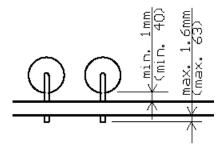
Fig. 6: Minimum and maximum distances when soldering THT gate resistors (in mm/mil)
