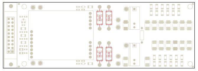
*Fig. 5: Assembly drawing of 2BB0108T with highlighted THT gate resistors Turn-on gate resistors: R120, R220 Turn-off gate resistors: R122, R222*
